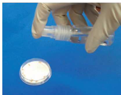
Fig. 12 Direct spray test method
