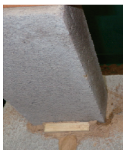
Fig. 10 No mud tubes built on treated concrete block in one week after installation
