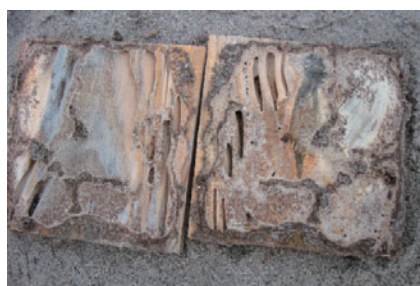
Fig. 4 Wood block damaged by termites on untreated soil
