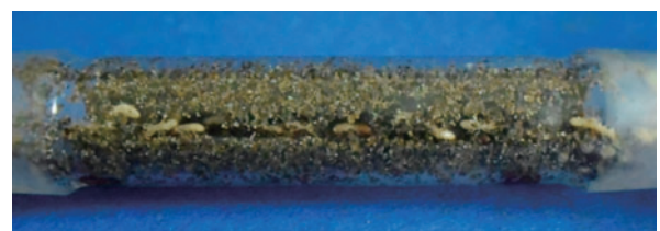
Fig. 2 Untreated 5-cm core soil penetrated by termites within one day exposure
