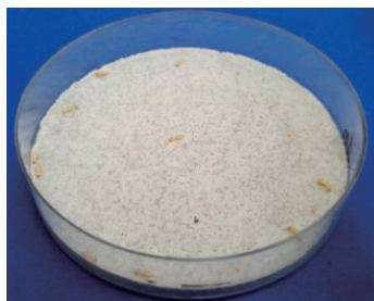
Fig. 6 Concrete plate contact test method
