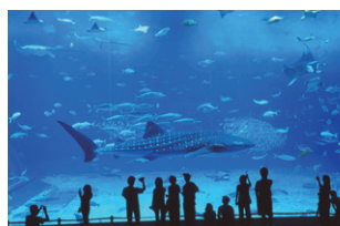
Large aquarium panel made of methyl methacrylate
