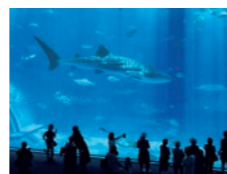
Large aquarium panel made of methyl methacrylate
